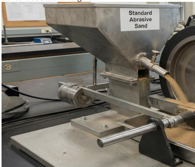
Fig. 2. Dry sand/rubber wheel abrasive test rig
